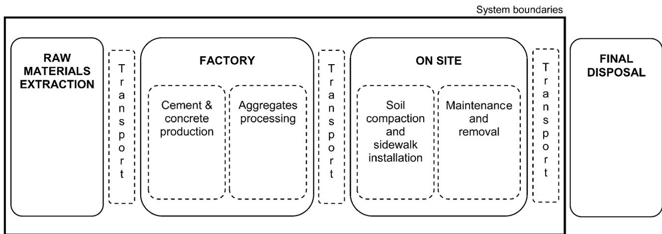
**Fig. 2** System boundaries and process chain under study
